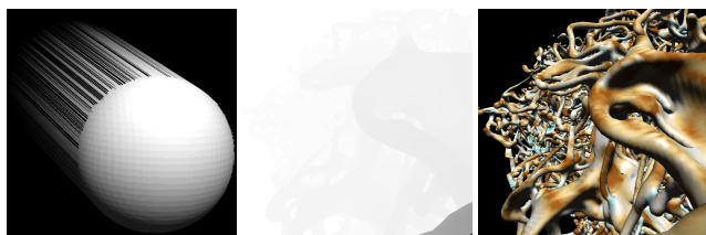
Figure 4: Left: Reprojection of a sphere showing “comet tail” artifacts caused by rubber banding to pixels on the far plane, which have not been correctly eliminated from the image. Middle/right: Depth map used for evaluating lossy depth compression and corresponding color image of a jet break-up in a non-Newtonian fluid in air (courtesy of ITLR, University of Stuttgart).
