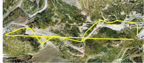
Figure 1: Path recorded showing significant location errors from the actual path (white area) due insufficient data collecting rate. But the almost straight yellow section fits rather well with the (slower) chairlift actual travelled path.
