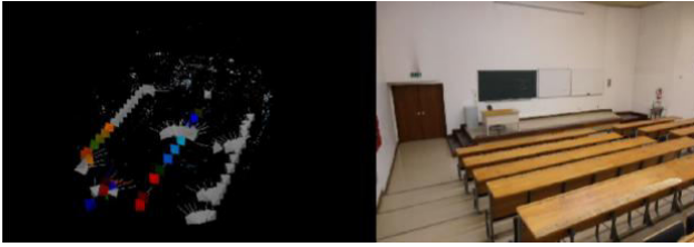
Figure 2. Example of an indoor reconstruction using VisualSFM (at the left). This structure represents an amphitheater (at the right). Analyzing the 3D structure recovered, few 3D points are visible and the structure semantic is hard to notice.
