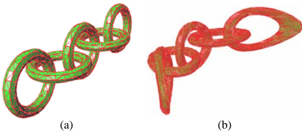
Figure 3: (a) The domain consists of 5 separated tori, which is of non-trivial topology. (b) The deformation of the object is achieved by bending the control net.
