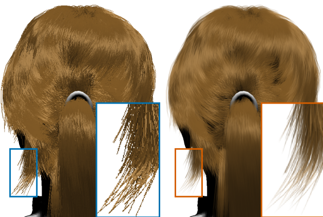
Figure 3: Kajiya-Kay shaded results from our strand rasterizer, on the left without any anti-aliasing, and with our coverage method on the right. A correct blending order is needed, since our calculation modifies the alpha channel (we use a PPLL to sort these fragments).
