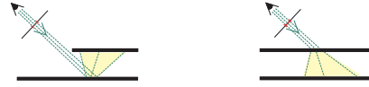
Figure 3: Because of rough reflection (left) or rough refraction (right) from the first surface, the light beam incident upon the second surface is no longer collimated even if the original light beam is.
