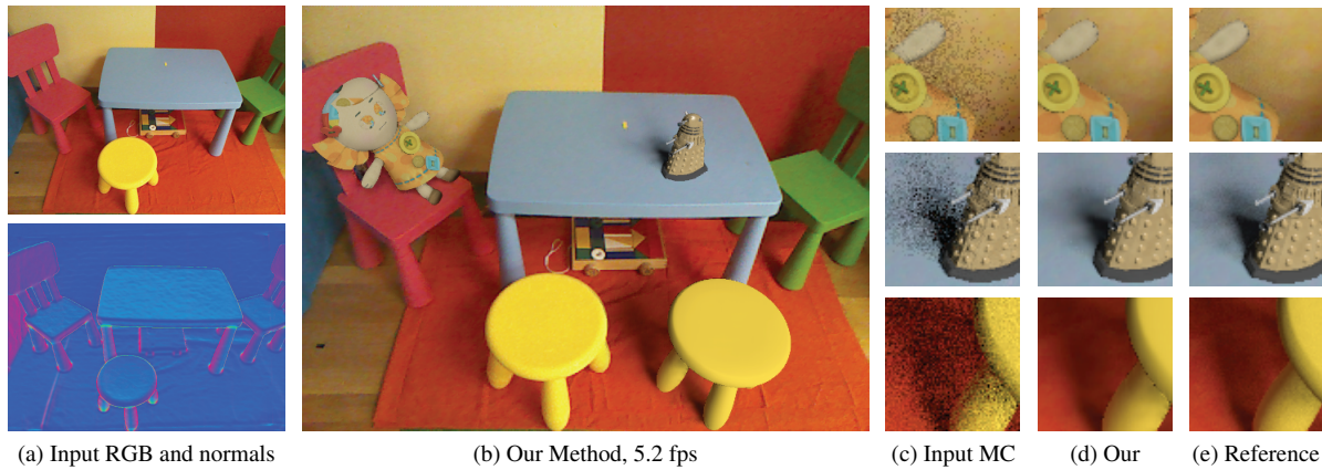
Figure 9: The PLAYROOM scene with input image and 3D reconstruction are shown in (a). We insert a virtual doll, toy robot, and a stool (the one on the right), with physically correct illumination, as shown in (b). We compare our result (16 spp, 0.19 sec) with unfiltered Monte Carlo (16 spp), which is very noisy, as well as reference (1024 spp, 12 sec) which is 60× slower.
