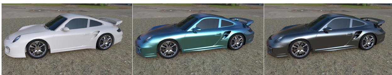
Figure 1: Renderings of car paints based on our micro-flake model. Left: pigment particles, Center: interference flakes, Right: mirror flakes.
