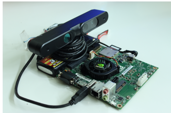
Figure 5: Jetson board connected to the ASUS Xtion depth sensor on top of a battery
