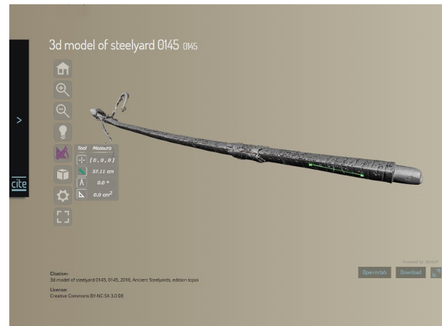
Figure 9: The measurement tool: by clicking on the panel icons the repository user can select four different interactive measurement tool: point picker, distance tool, angle tool, area tool (example available at http://repository.edition-topoi.org/collection/BSYP/single/0722/0 ).
