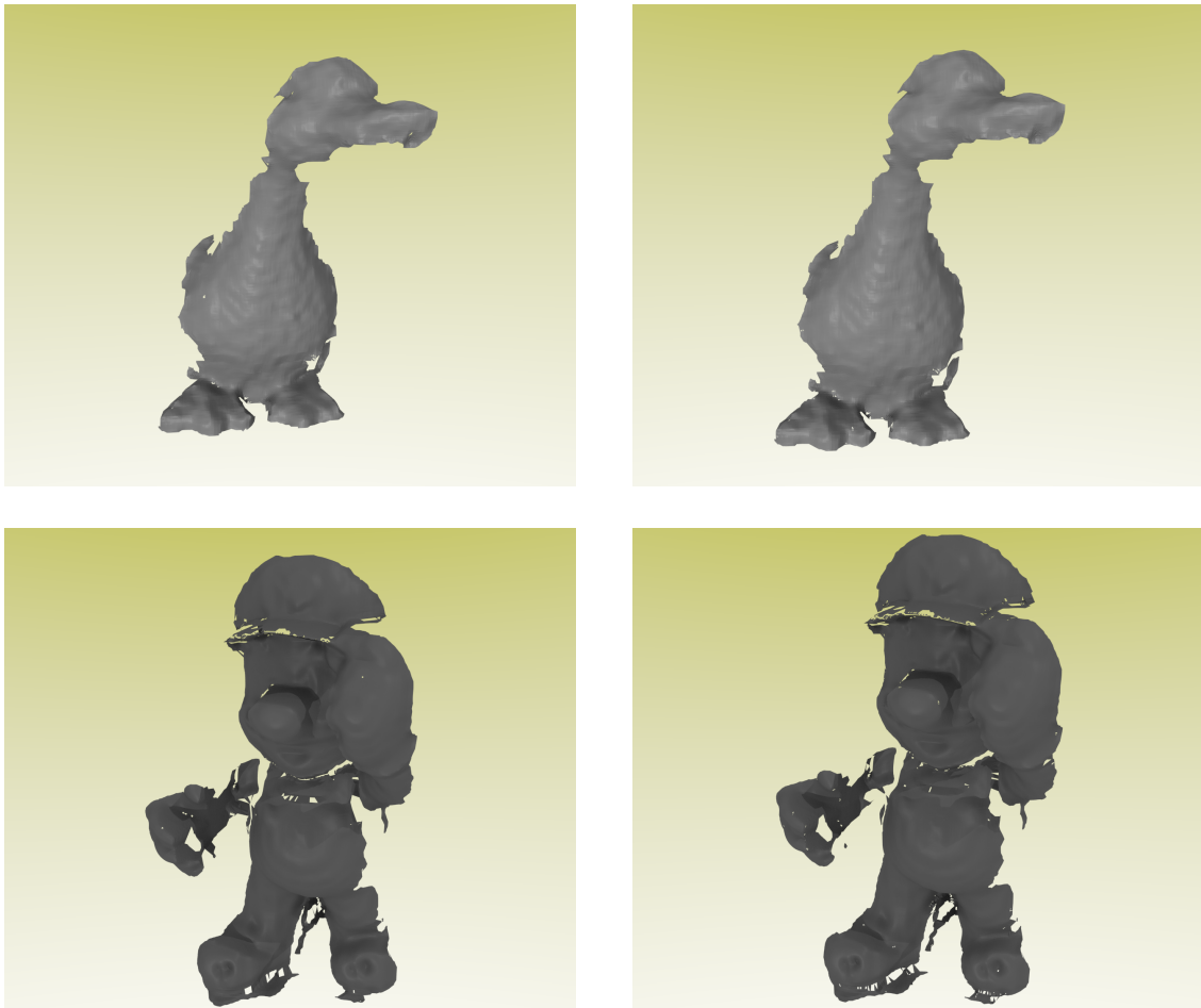
Figure 8: BPA (left) and RBPA (right) reconstruction using our radius estimation. Note the equivalent level of detail.
