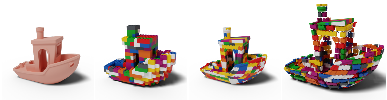
Figure 1: From left to right: the original model, the LEGO bricks placed according to the layout, and the resulting custom bricks, an exploded view of the custom bricks.
