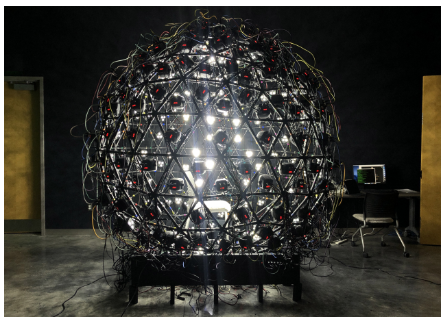
Figure 2: VarIS with all white lights activated.
