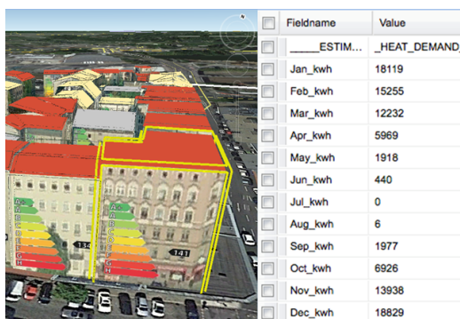
Figure 1: Visualization of estimated heat demand values of a building in Berlin. The screenshot is retrieved from 3DCityDB Webclient developed by TU München [YSKK14]
