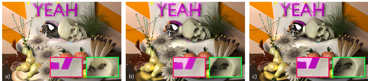
Figure 1: Screen space methods for indirect illumination [NRS14a] (left) not only underestimate effects of invisible geometry (left inset), but also routinely ignore visibility (right inset), which is added by our approach (middle) to produce results similar to a path-tracing reference (right). Our approach renders this scene with 202 k triangles in 65 ms (768×512 px.).
