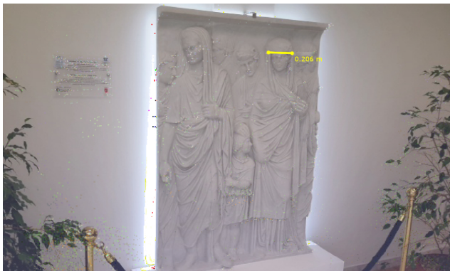
Figure 1: Metric measurement of an Ara Pacis Flamini's frieze (marble copy for public display) acquired by our system. The measurement has been taken by the user on the reconstructed 3D point cloud and returned to display in metric dimension. The average error compared to ground truth is 2.8%.
