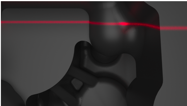
Figure 12: Rendered laser line with speckle pattern.
