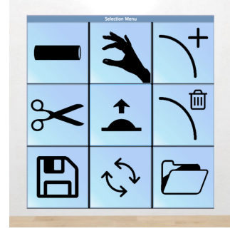
Figure 3: The menu for selecting the editing tool. From left to right, top to bottom: new starting rod (requires a reset of the scene); deformation tool; add rod tool; cutting tool; extrusion tool; erase rod tool; save scene; reset to empty scene; load scene from file.
