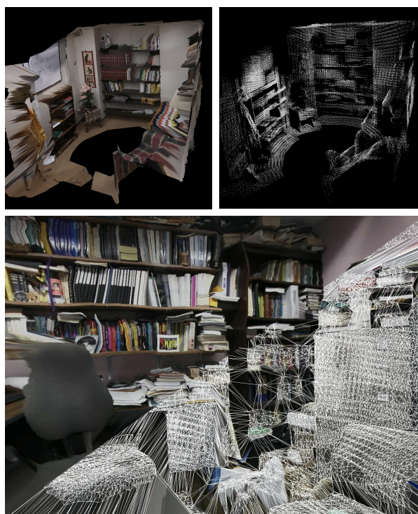
Figure 1: The room in the two top images and the room in the bottom image are each modeled with a single depth enhanced panorama. The depth enhanced panoramas have 299,820/169,083 triangles and each was acquired under 30 minutes with a $3,000 device.
