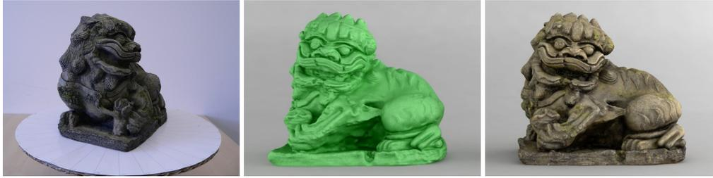
**Figure 2.1: Dragon statue.** Left: Notice the amount of micro-details that are present on the surface of this model. Center: Geometry of the 3D scanned reconstruction; Right: Colored 3D rendering of the reconstructed 3D model. Courtesy of Augmented Vision department at DFKI.
